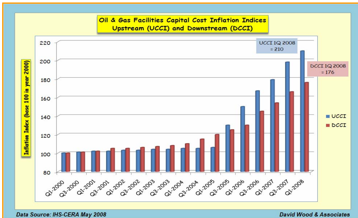
Figure 4.2.3. Oil and gas industry cost inflation trends for upstream (UCCI index of IHS-CERA) and downstream (DCCI index of IHS-CERA) show costs worldwide have doubled since 2000 and continue to increase in 2008. Source: David Wood, World Oil Feb 2008.
